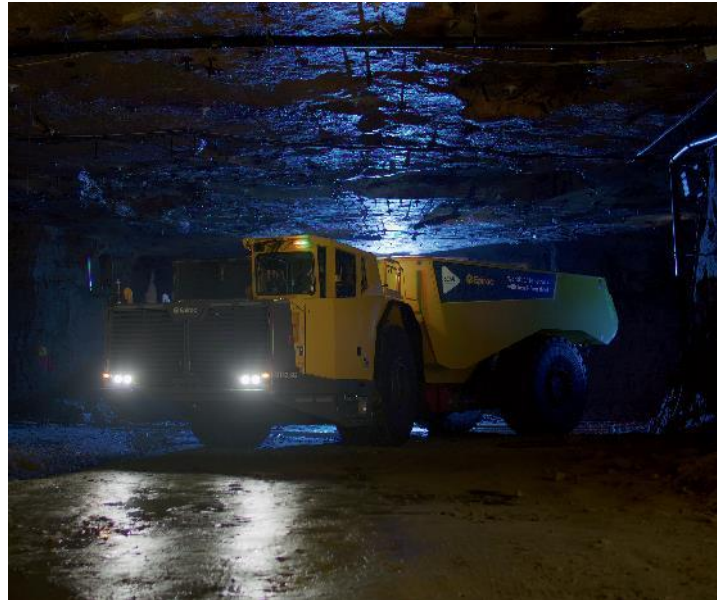
A battery-electric Minetruck MT42 with a dump box made of fossil-free steel, thereby reducing CO 2 e emissions by 10 tonnes per manufactured dump box.
