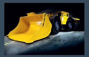
In Australia, Epiroc and Newcrest Mining have successfully managed to deploy one of the first underground autonomous mixed-fleet solutions in the world at a major block-caving mine. Not only the Epiroc ST18 loaders are autonomous, but also the machines from another equipment supplier. The underground conditions are demanding. The fully autonomous and unmanned loaders are targeted to run 25–26 km/h speed underground, while having only 30 cm margin to the sharp hard-rock tunnel walls on each side.
