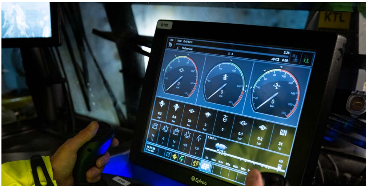
The Boltec rock bolting rigs M10 S and E10 S are designed to give increased productivity and bolt installation quality thanks to intelligent options and compatibility with different bolt types. Thanks to a new operator control panel, reduced noise levels and better visibility, operator ergonomics are also improved. The battery-electric versions are indicated with SG in the model name, which stands for Smart and Green - Boltec M10 SG and Boltec E10 SG.
