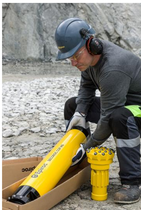
The new M-series down-the-hole hammers that are shorter, lighter and faster compared to its predecessors.
